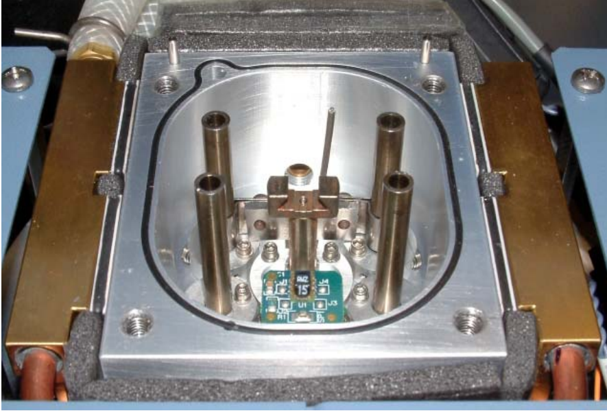
Figure 18 DMA-RH sample chamber installed properly.
