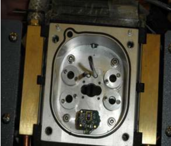
Figure 12 Mounting collars installed.
