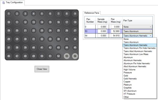
Select the position that you'd like to place your reference pan. Do not delete any of the reference pans already in place unless you are replacing it due to contamination or if the pan was damaged or lost. The selected position will highlight grey and a new line will appear in the table. Ensure you enter the mass of the pan that was recorded and choose the correct pan type from the dropdown menu.
