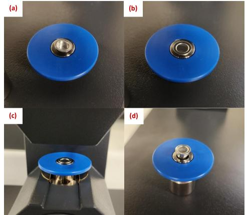
Immediately place the pan into the autosampler and enter the details in to the software as seen in <u>Setting up a</u> run. Ensure you match the reference and sample pan types. See <u>Reference pans</u> for more info.
