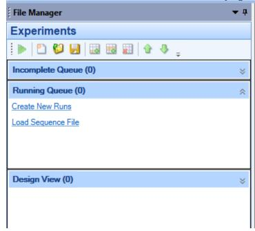
Click on **Create New Runs** to add a run. You should see the following in the middle of the **Experiments** window. Enter the **Sample Name** and the corresponding **Pan Number** you wish to place the sample in. Choose the **Pan Type**. See the section on <u>Loading and choosing pans</u> for more info. You may optionally enter a **Project** and all the filenames generated will have the project name in them automatically as seen in the example.
