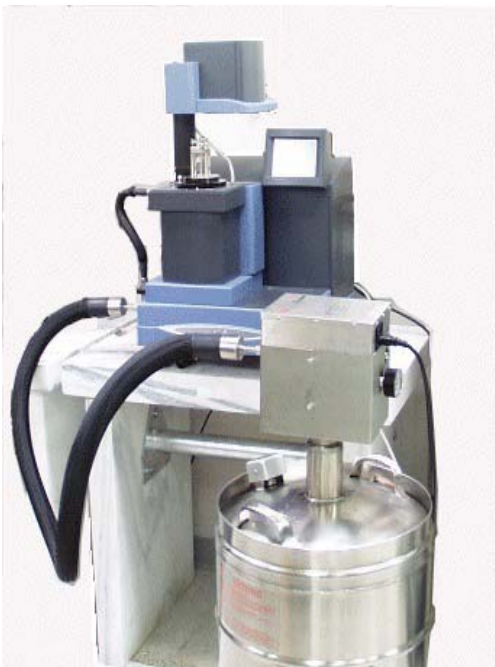
Figure 13 GCA attached to DMA Q800 (bulk source not shown).
