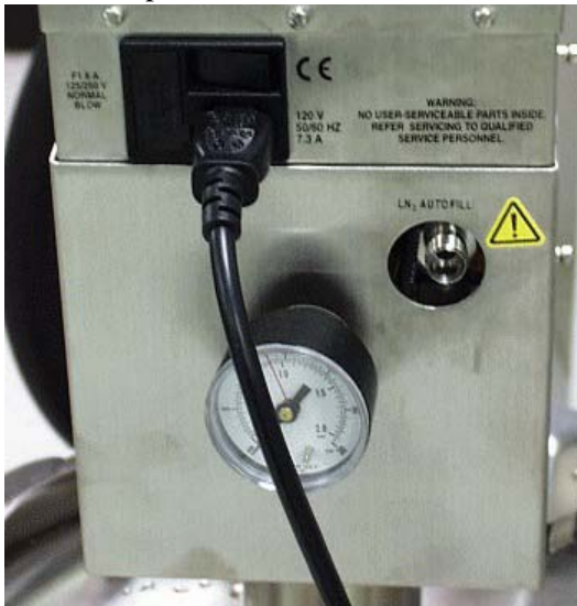
Figure 19 Power cable attached.
