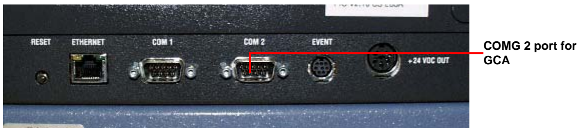
Figure 10 DMA Q800 ports on left rear.
