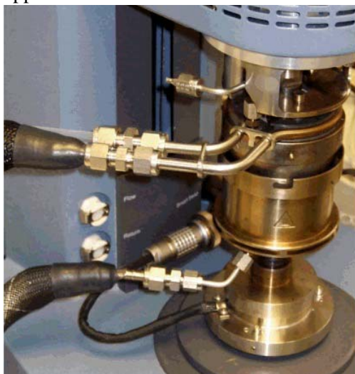
Figure 15 Coolant transfer hose connected to upper and lower coolant inlets.
