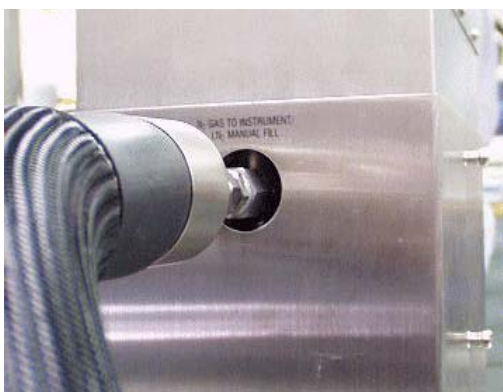
Figure 14 Coolant hose attached to fitting.
