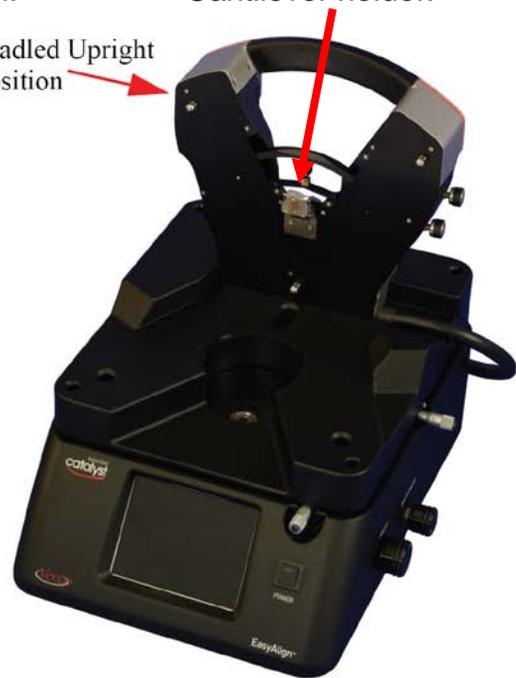
**AFM Head mounted on microscope stage.**
